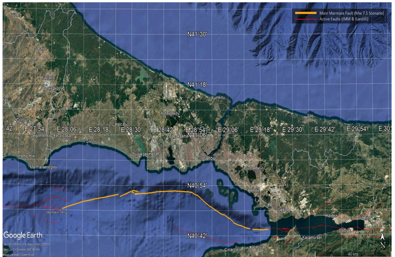
Figure 1. Tectonic setting of the Sea of Marmara showing the active fault system (thin red lines) and the assumed rupture trace for the deterministic Mw 7.5 earthquake scenario (thick orange line) based on the IMM and Kandilli dataset (Map base: Google Earth Pro).
